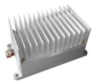
The built-in dynamic power sensor in SmartAmp<sup>™</sup> adjusts the Radio Frequency (RF) power output level by reading the input signal power. This Automatic Gain Control (AGC) Technology, Teletronics' patented technology effectively making the RF amplifiers "Plug & Play" delivers the maximum output power at various input levels while keeping the distortion at a minimum.
